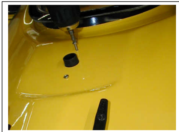
Fig. 9 – Installation of Trim Tab assembly.
