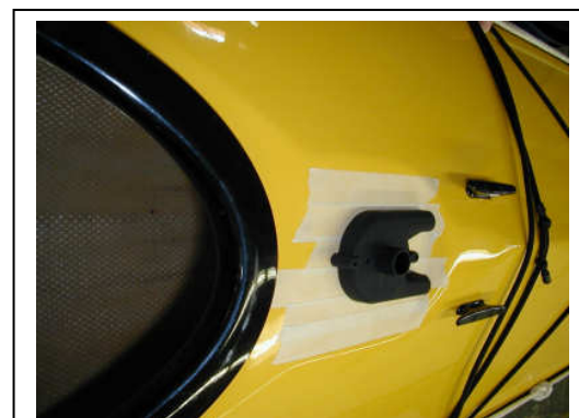
Fig. 4 – Trim Tap placed atop masked area.
