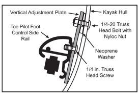
**fig. 1.** Cross-sectional view of mounting Toe Pilot Foot Control using Vertical Adjustment Plate.
